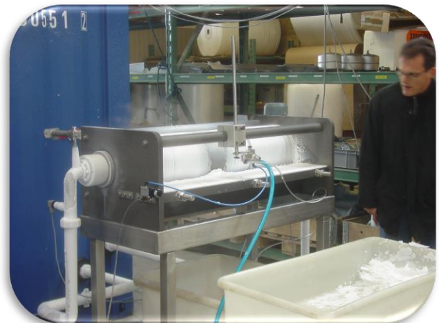
Shock freezing of cellulose fibers. -80°C plant
